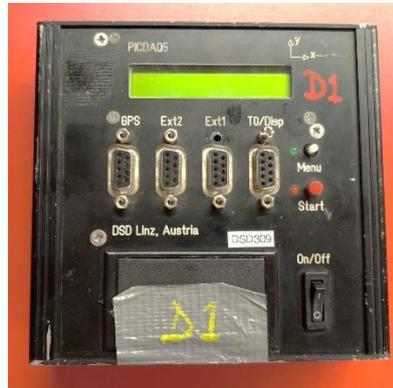
**Fig. 5.** Data acquisition platform - PicDAQ 5.
