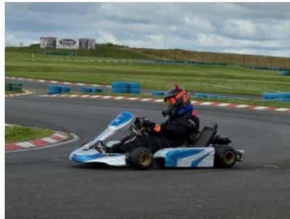
**Fig. 7.** U.O. Kart with Ground Effect fairing
