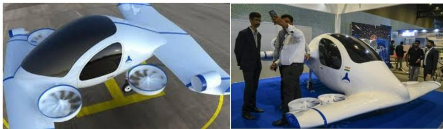
Fig. 6. a), b) Flying taxi with two pairs of wings and orientable electric propellants, [4].
