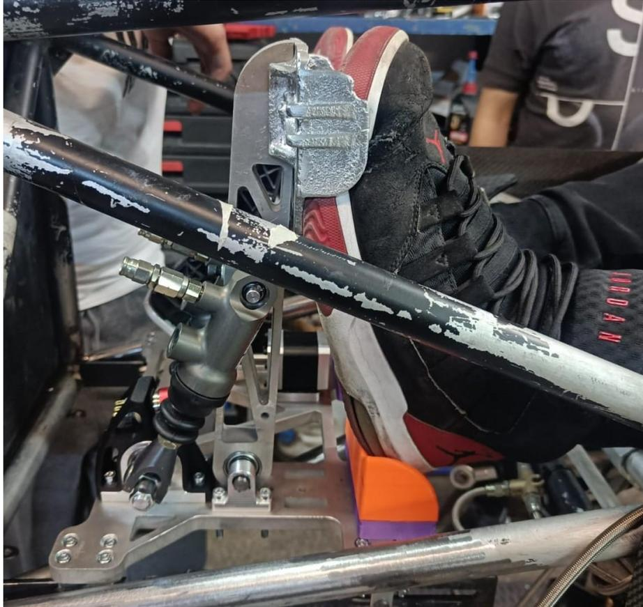
**Fig. 13.** Photo of one of our drivers inside the single seater to test the of the pedal box
