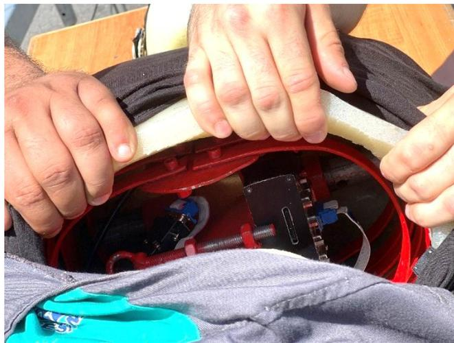
**Fig. 6.** PicDAQ 5 mounted inside the dummy's thorax
