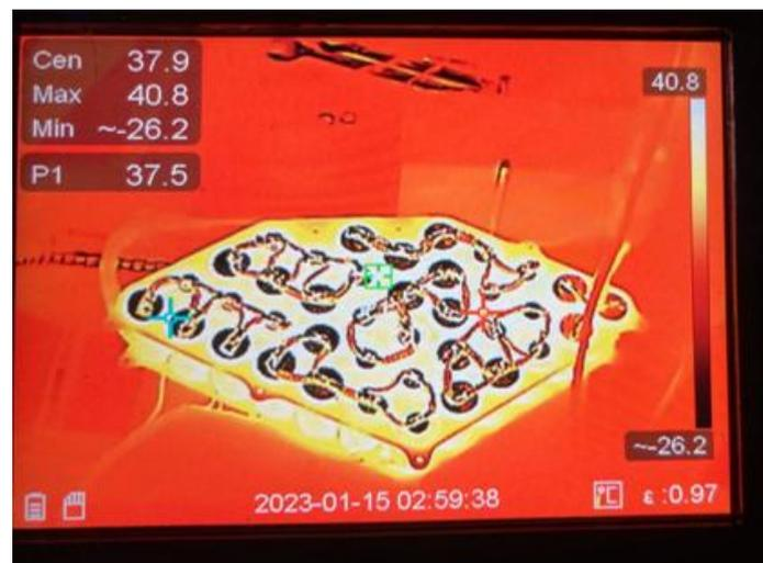
**Fig. 7.** Battery pack temperature heat distribution at the end of the test.
