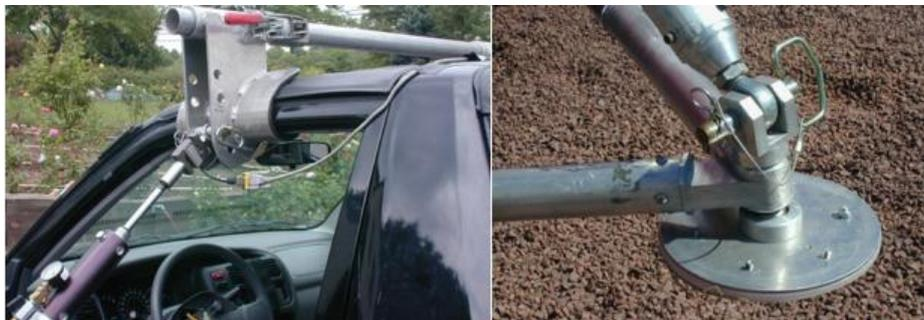
**Fig. 6.** Schematic of a modern outrigger system with adjustable height and low-inertia rollers [4].
