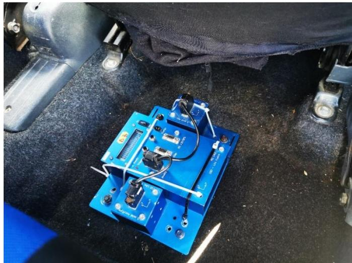
**Fig. 8.** PicDAQ 4 mounted inside the vehicle.
