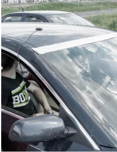
**Fig. 4.** Antenna mounted on the vehicle roof
