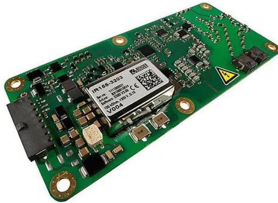
**Fig. 4.** Bender A-ISOMETER® IR155-3204 Insulation Monitoring Device.
