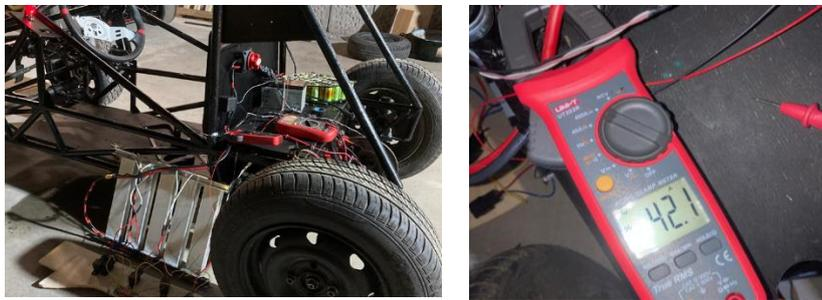
**Fig. 6.** 0.9-ohm resistive power load test setup.
