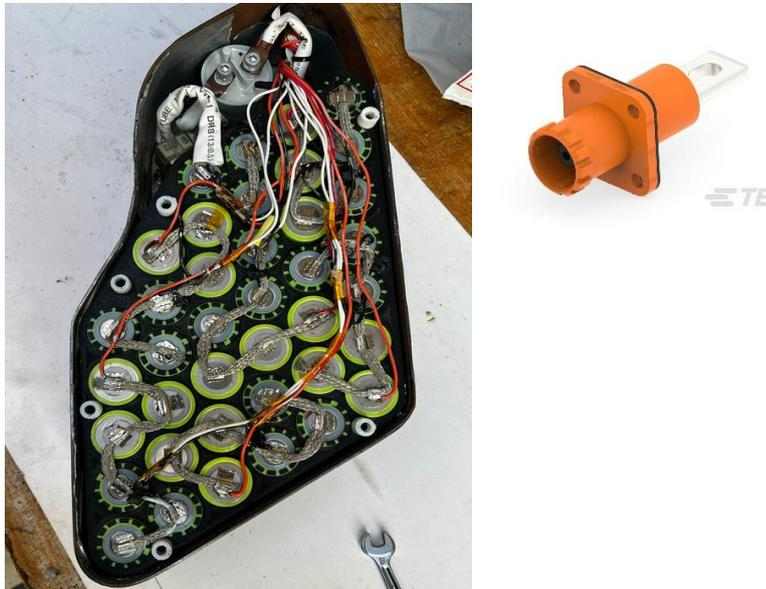
**Fig. 4.** Assembled pack with thermistors and cell voltage readout cables, high voltage terminal.
