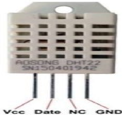
Figure 4.2. Humidity transducer (from [4])
