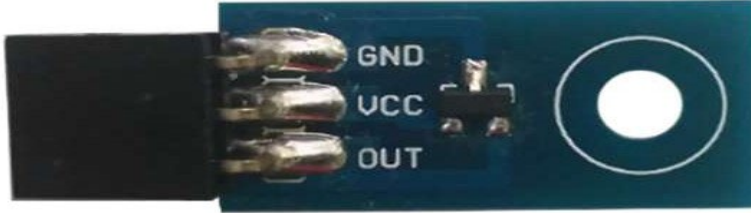
Figure 3.2. Temperature Transducer LM50 (from [5])
