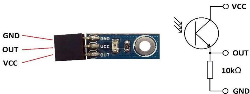
Figure 5.9. Analogic Light Transducer (from [1, 2], [7])
