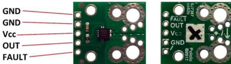
Figure 7.3. Current transducer (from [1,2])
