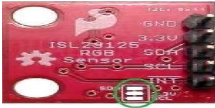
Figure 5.14. The use of the step up to 1 resistor (from [1],[7])
