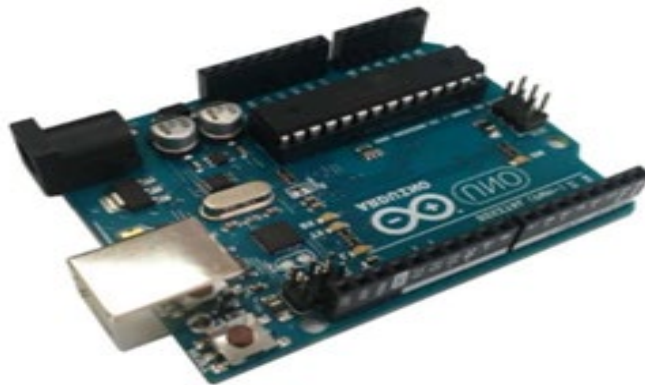
Figure 1.1 Arduino Uno Development Board (from [1])
