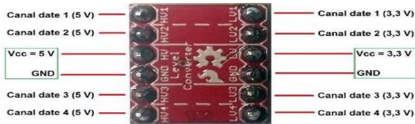
Figure 5.15. The bidirectional logic level convertor (from [1, 2], [7])
