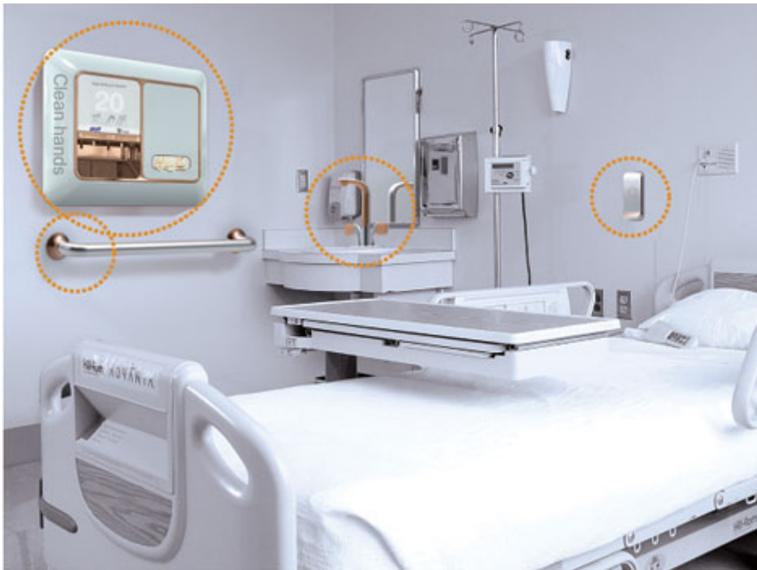
Figure 3.15. Hospital room with sani-station and touch-point hardware: grab bar, faucet, and light switch.
