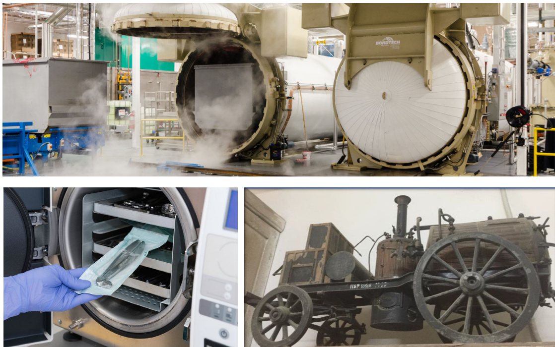
Figure 4.8. Autoclaves for thermal medical waste treatment and instruments disinfection compare with a steam equipment in Romania used in First World War After treatment, the disinfected waste is usually compacted. It can then be sent to a landfill or to a waste-to-energy facility, depending on local regulations and the treatment chain used by the operator.
