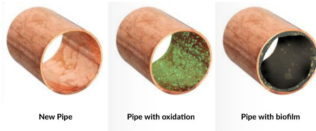
Figure 3.25. Surface oxidation of copper can lead to surfaces with increased roughness increases, which in turn, can contribute to increased corrosion and scaling. As corrosion and scaling become more pronounced, they lead to more significant biofilm development.
