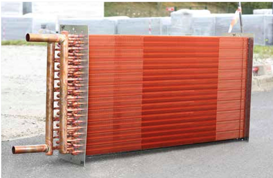
Figure 3.22 Copper coil air handling unit for harnessing the antimicrobial properties of copper in hospital applications, manufactured in Europe by French manufacturer Hydronic.
